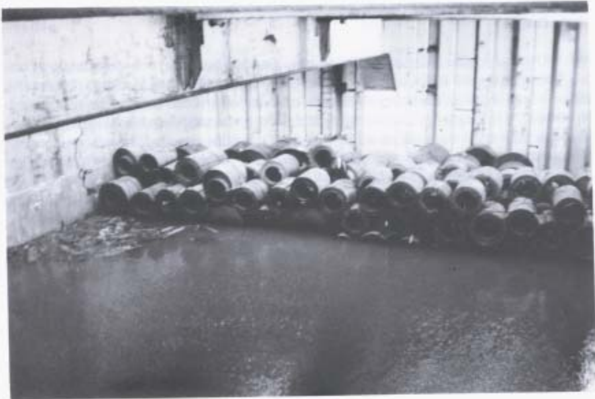
Photograph A Poorly secured coils in flooded hold
