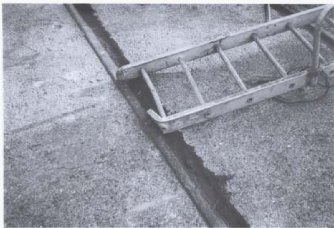
Photograph 4 Damaged foot of the ladder
