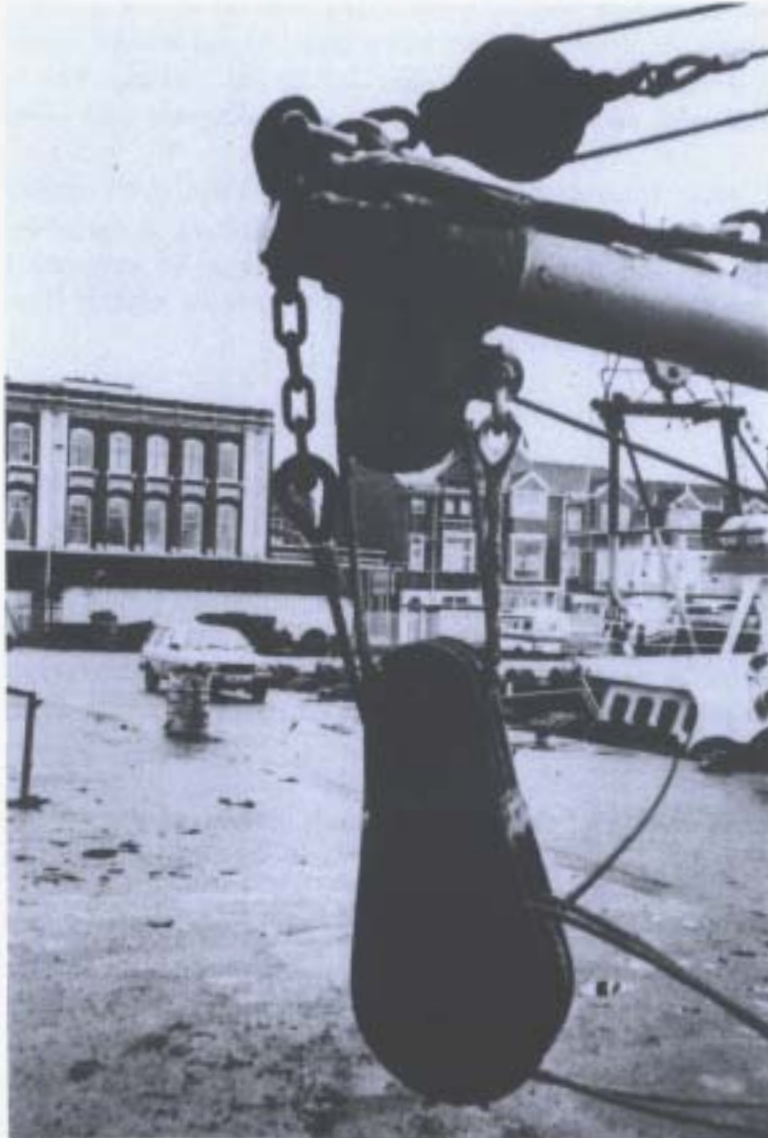
View of double purchase block in normal position with new quick release wire fitted. Note: the ferrule has been replaced by a "traditional" splice.
