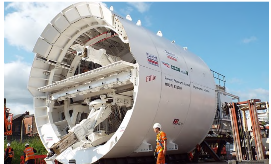
Open Face Tunnel Boring Machine
