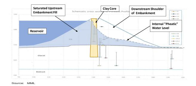
Figure. B6 Measured phreatic water levels within the embankment
