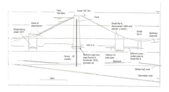
**Figure C2. Section showing location of grout curtain various investigation and monitoring shafts (**Based on British Waterways Drawing HH /BWB /02/03, 1984)
