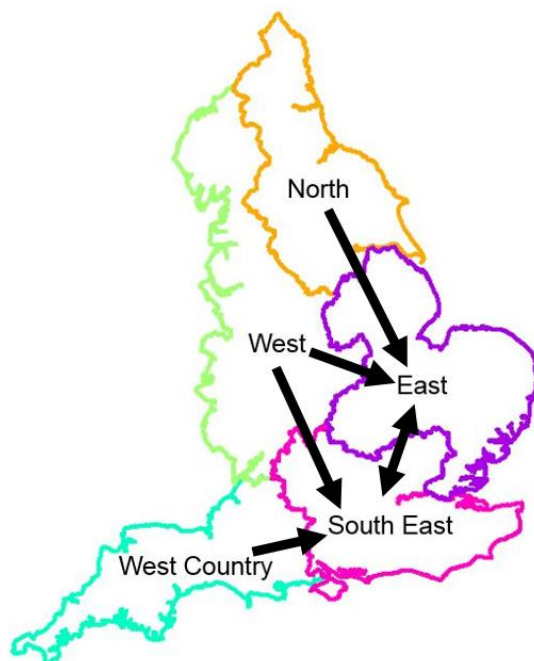
Figure 24: Inter-regional transfers that occur most commonly in all of the ‘efficient’ solution portfolios above the inflection points on the trade-off fronts for the low, central and high demand scenarios, under the possible transfer search model configuration (see points a, b and c on figure 23).
