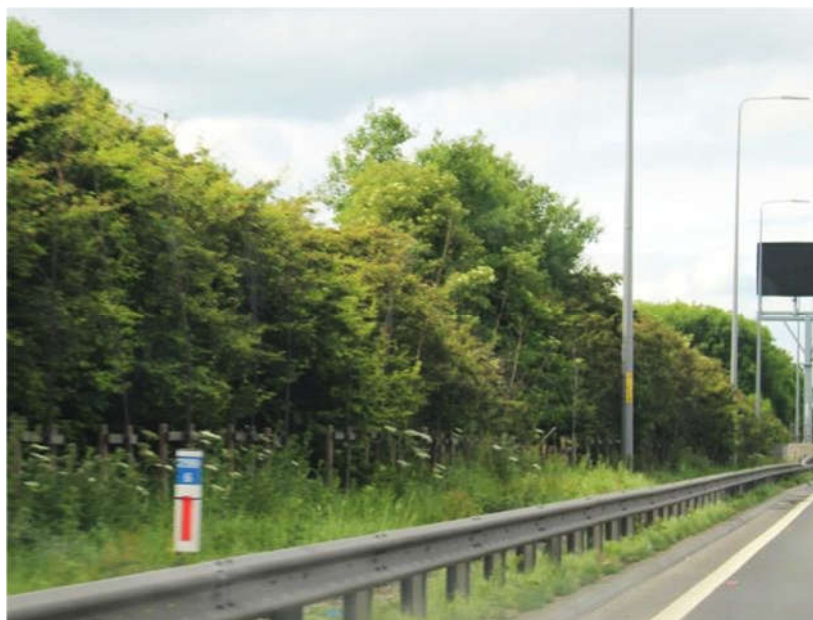
Figure 5-10 Standard tree avenue at rear of verge and in front of existing mature hedge
