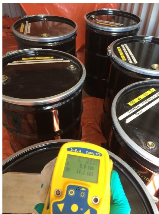
Figure 7 Storage of drummed radioactive materials in a secure container
