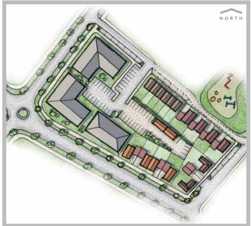
Indicative sketch for a 1ha medium density residential area, showing building, street and parking layouts
