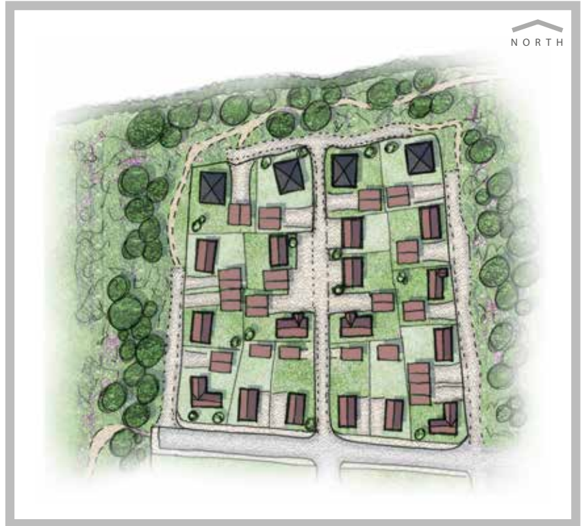
Indicative sketch for a 1ha very low density residential area, showing building, street and parking layouts
