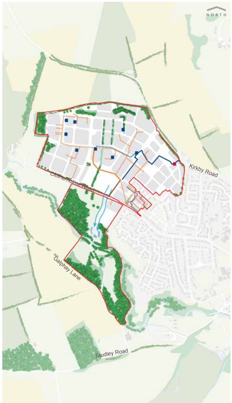
Proposed surface water management features and utilities
