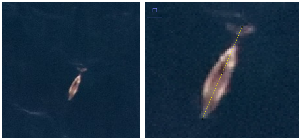
Figure 6 Example of a good quality image (grade 1) measured in ImageJ. Left: image extent, right: zoomed in showing measurement points for length.
