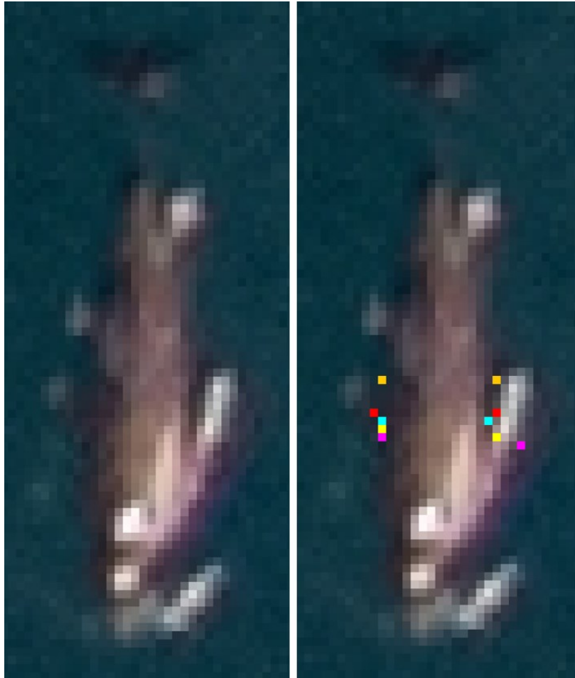
Figure 37 Animal 2: Location of pixels identified by the multiple users as the width points of measurement. Difference in width measurement: 8.0 cm.
