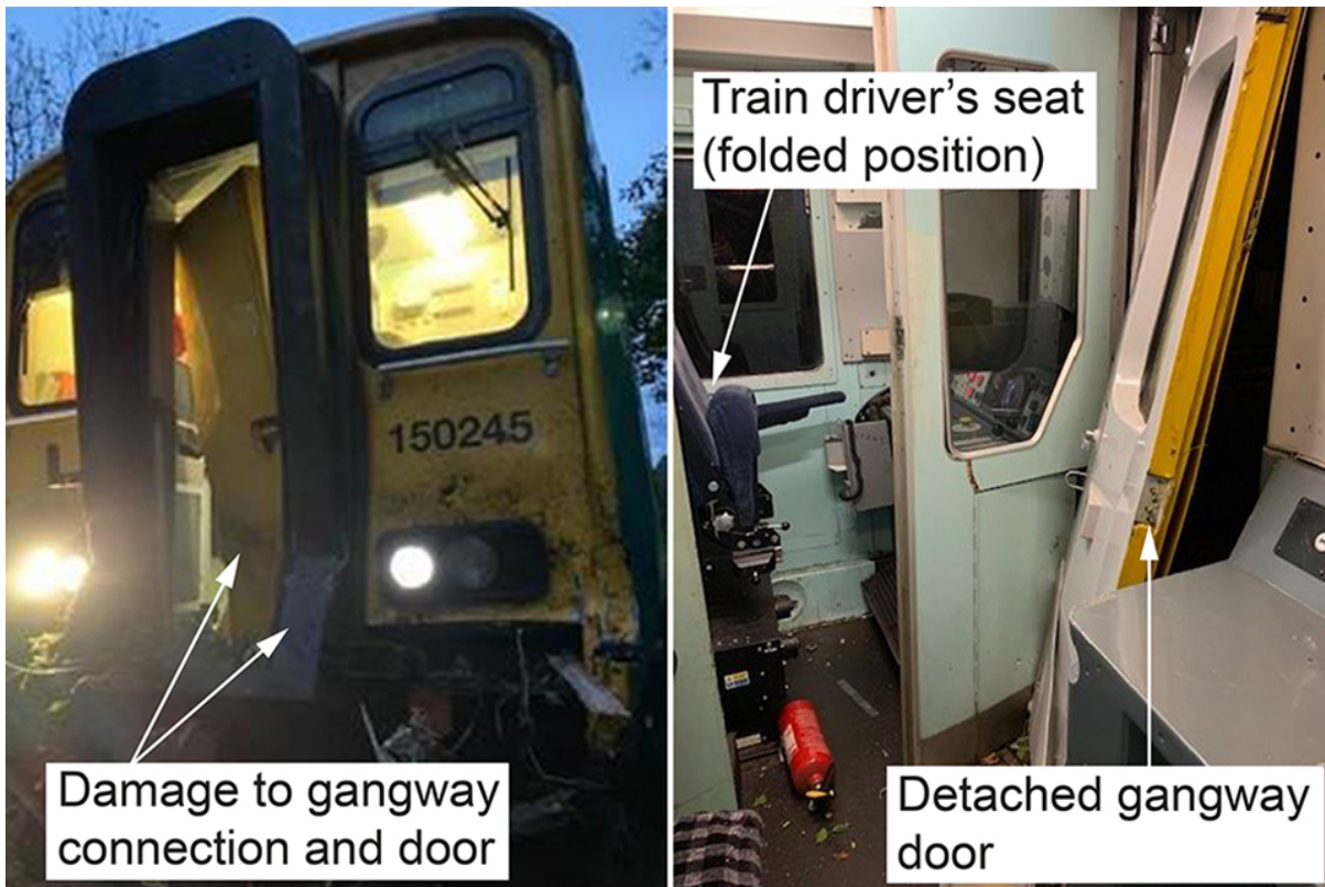
Damage to the train front and driving cab area (images courtesy of Network Rail)
