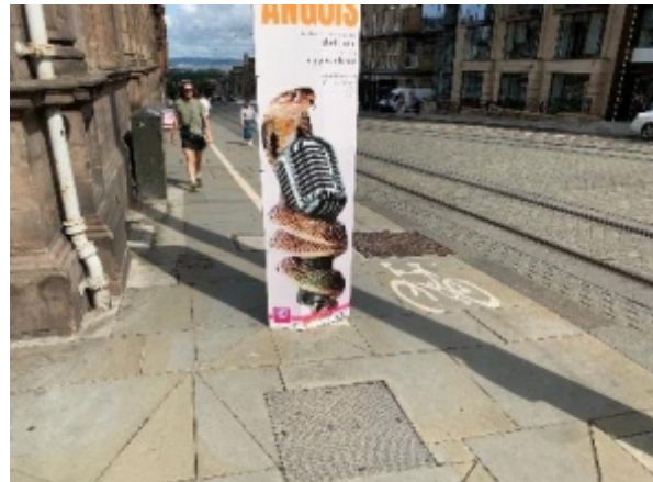
Start of parallel footway and cycleway, separated only by a painted line and with no tactile threshold
