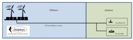
Case 2. Offshore floating wind farm with a centralised electrolyser vessel and export pipeline to shore
