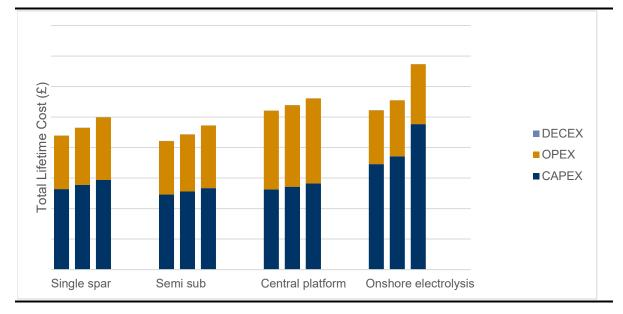
As can be seen above, the semi-sub provides the most cost-effective solution. Both the integrated spar and semi-sub design are preferable to the options where electrolysis takes place on a single offshore platform/vessel or onshore.
