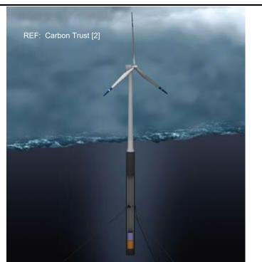
Figure 2.2 HyWind Spar Sub-structure Design
