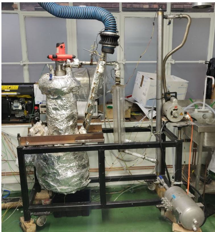
Figure 4 - Assembled system; reactor, gas outlet, burner exhaust, condenser, liquid collection line, vacuum pump
