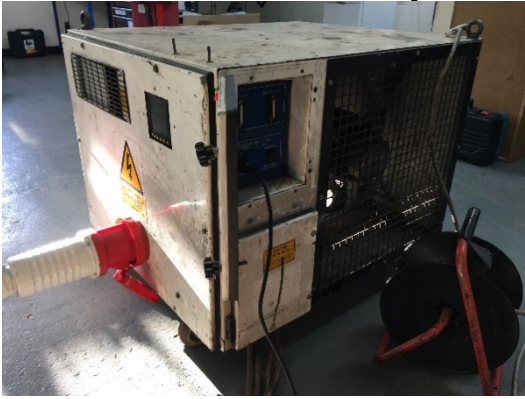
Figure 25 - 100kW load bank
