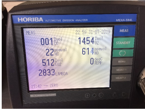
Figure 45 - EN590 diesel emissions
