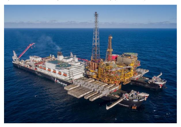
The SLV was stationed beneath the topside and the 16 large beams of the TLS (paired into 8 fork-lift units) were positioned under the prepared lift points on the underside of the PGDS (Figure 17). Each fork-lift unit had a yoke (lifting pad) that fitted on to one of the topside lifting points and was kept positively in touch with the topside by a hydraulic system that compensated for the movement of the vessel.
