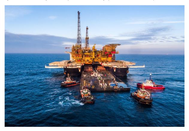
Figure 26. Transferring the Brent Delta topside from the *Pioneering Spirit* to the *Iron Lady*.
