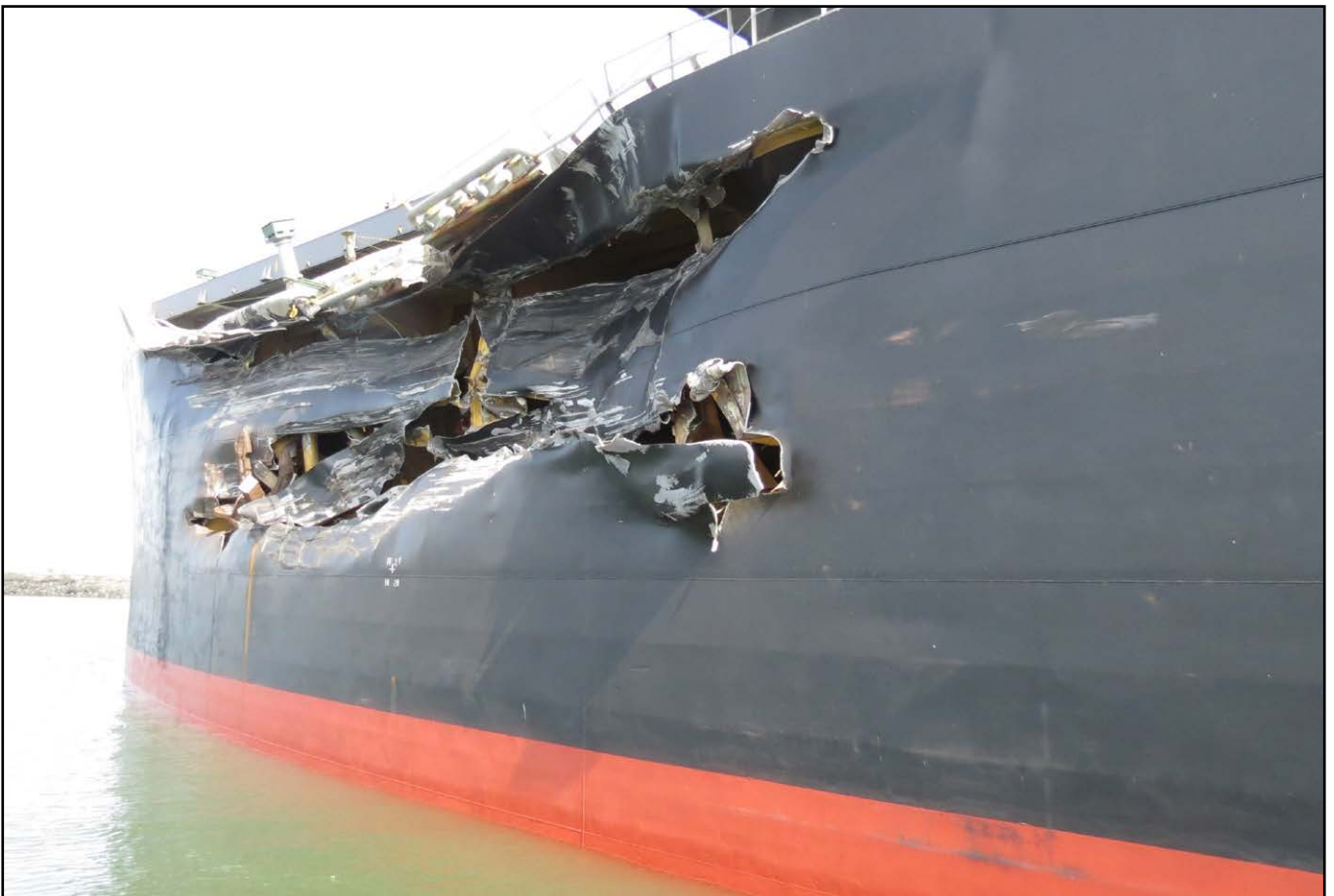
Figure 6: Damage to port side of Cape Mathilde
