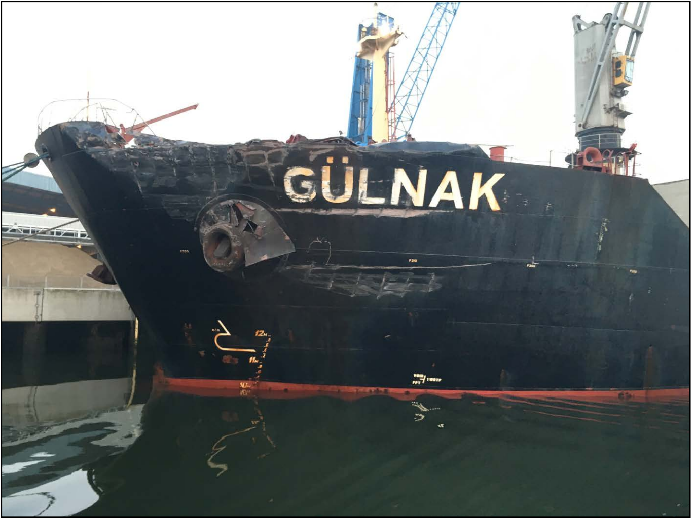
Figure 5: Damage to port bow of Gülnek
