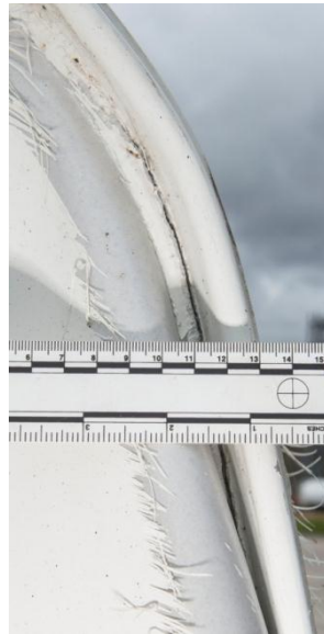
Figure 14 GRW tanker J2580 – rupture in the weld at top of impact zone
