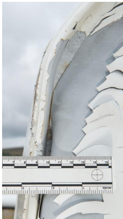
Figure 16 GRW tanker J3910 – rupture at toe of weld at top of impact zone
