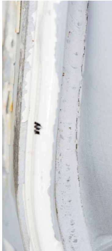
Figure 17 GRW tanker J3910 – crack at toe of weld at bottom of impact zone
