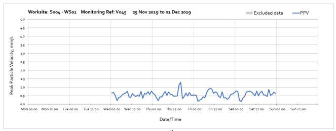
Note: the vibration monitor was installed on the 25<sup>th</sup> of November. The high variability in vibration levels inside and outside construction hours were mainly due to road traffic generated vibration rather than being attributable to HS2 constuction works.
