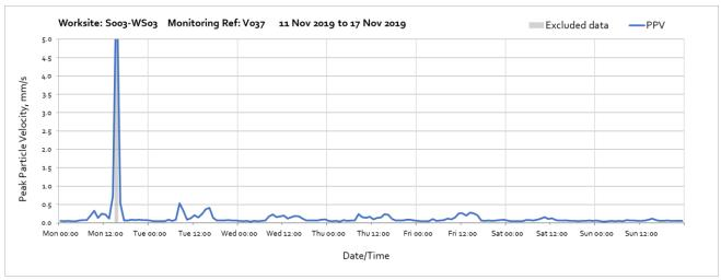
Note: High vibration levels at 11:00 on Monday 11<sup>th</sup> November were due to local disturbance of the vibration monitor and are not representative of HS2 vibration levels.
