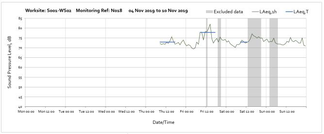
Note: Missing data until 08:00 on Thursday the 6<sup>th</sup> of November were due to a power failure at the monitoring station.
