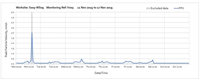
Note: High vibration levels on Monday the 11<sup>th</sup> of November were due to local disturbance of the vibration monitor and are not representative of HS2 vibration levels.
