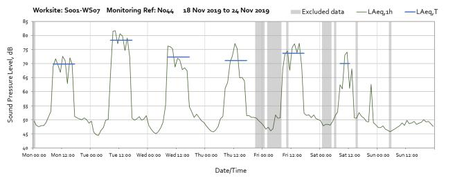
Note: Noise levels above the SOAEL on Tuesday the 19<sup>th</sup> and Thursday the 21<sup>st</sup> of November were due to noise from dust suppression equipment installed in proximity to the monitor. Considering distance attenuation noise levels would be below the SOAEL at the nearest receptors to the works.
