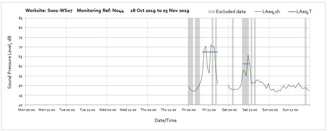
Note: Missing data between 18:00 and 23:00 on Friday the 1st of November were due to a power failure at the construction site.
