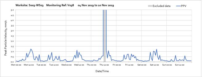
Note: High vibration levels between 12:00 and 15:00 on Thursday 7<sup>th</sup> November were due to local disturbance of the vibration monitor and are not representative of HS2 vibration levels.
