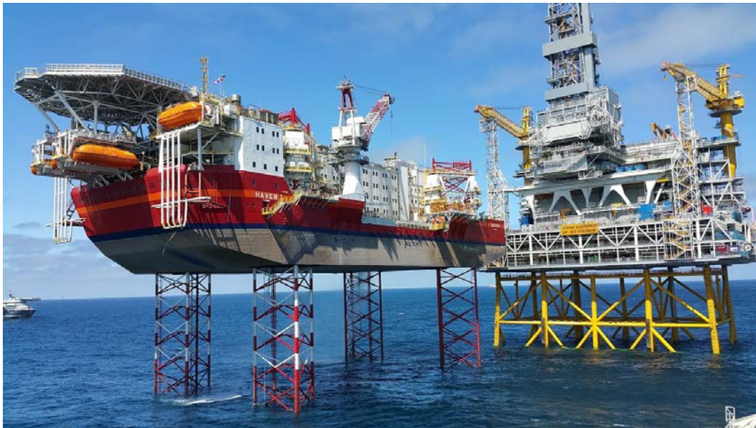
Figure 3: Master Marine's jack up: The Haven 18
