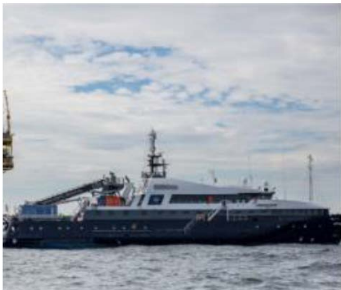
Figure 5: Image of a walk to work vessel'
