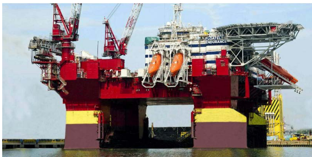
Figure 2: a semi-submersible accommodation support vessel
