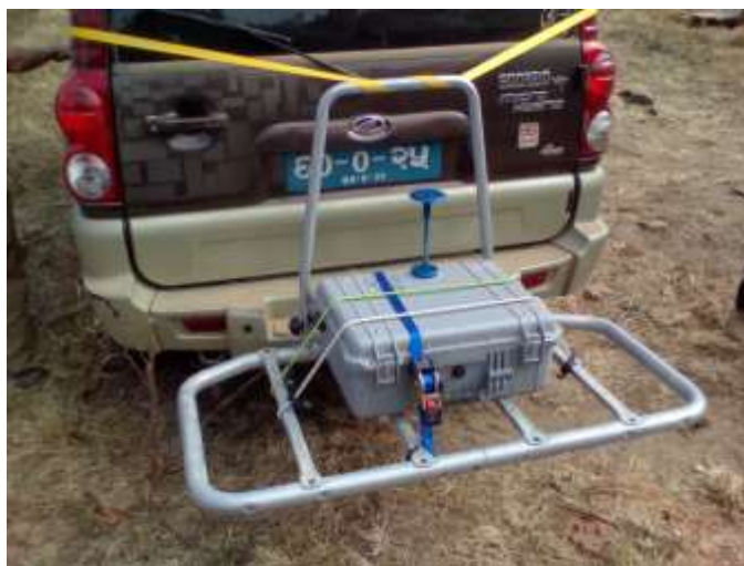
Figure 23 Enclosure fixed to vehicle rack
