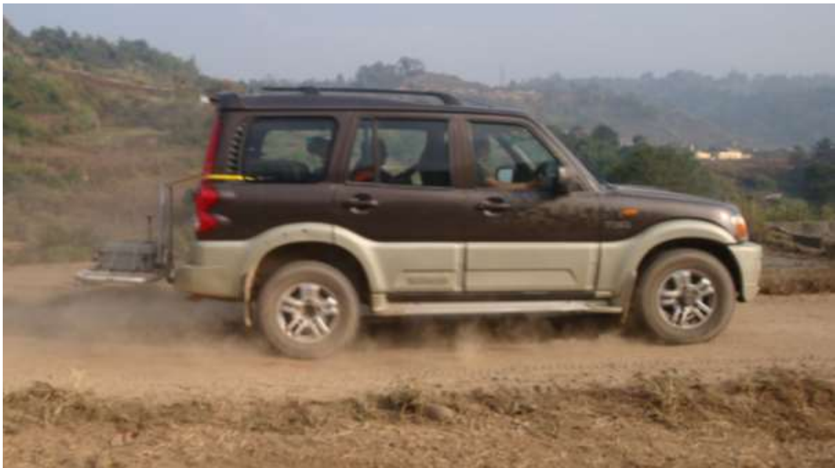
Figure 1 Dust equipment attached to vehicle
