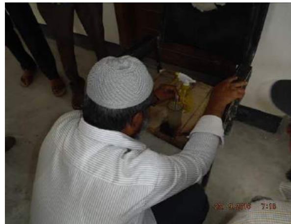
(b) Testing chloride content of water using Quantab Strips at Rampal
