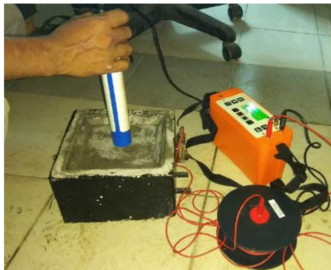
Figure 4-14 Half-cell potential testing on a concrete ponding slab
