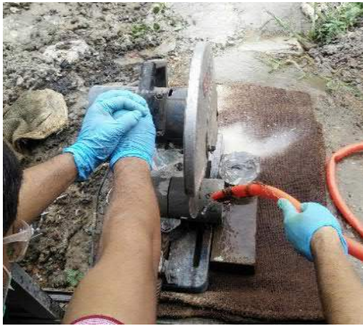
(a) Concrete saw cutting
