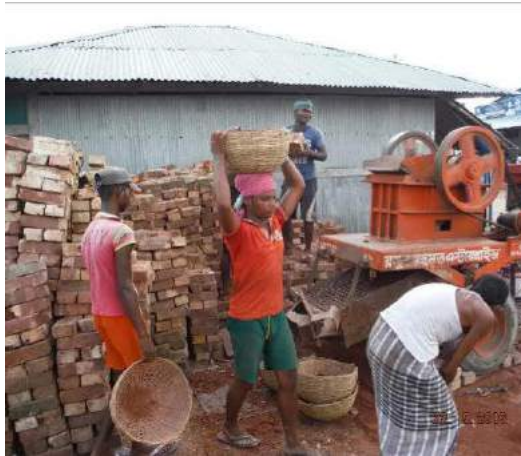
(a) Machine crushed brick aggregates
