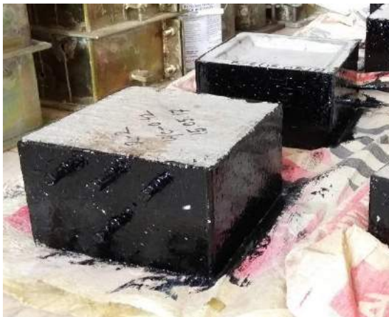
(d) Epoxy painting of side faces and exposed length of rebar
