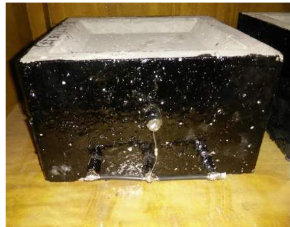
(e) Top and bottom rebars connected with 100 Ω resistor
