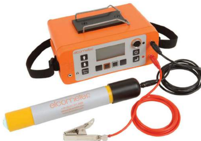
Figure 3-4 Elcometer 331 Half-cell meter with silver in silver chloride reference electrode
