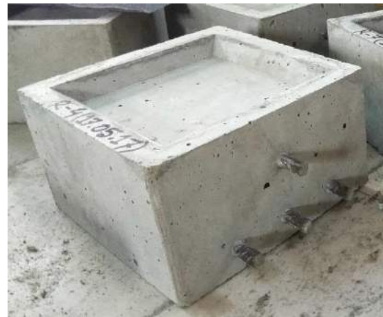
(c) Demoulded concrete slab showing ponding reservoir on the top
