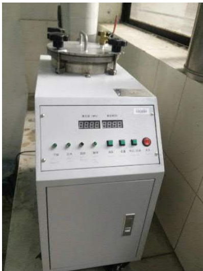
(c) Concrete vacuum saturation apparatus
