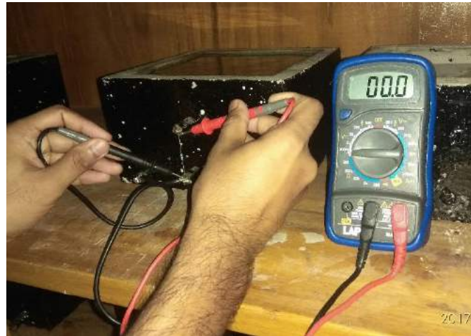
Figure 4-13 Measurement of macro-cell corrosion on ponding slabs
