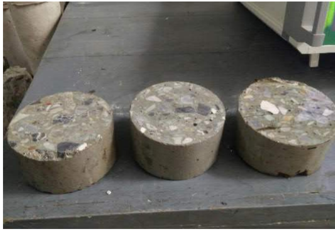
(b) Concrete specimen 100mm diameter and 50mm height
