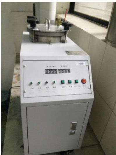
(c) Concrete vacuum saturation apparatus
