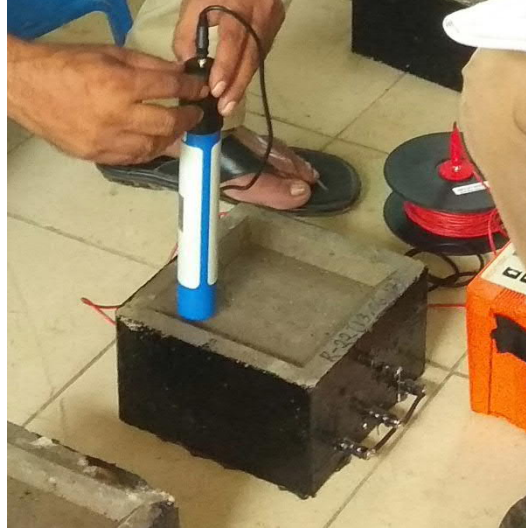
Figure 14 Half-cell potential testing on a concrete ponding slab
