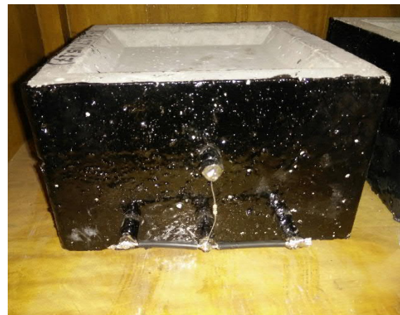
(e) Top and bottom rebars connected with 100 \Omega resistor
