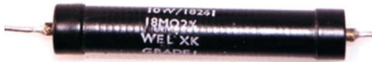
d Wire-wound Resistor Inscribed 18\text{ M}\Omega
