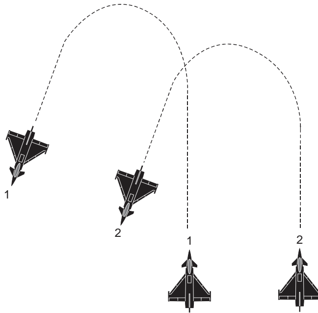
8-21 Fig 23 Variable Delay Turn 160° Left
