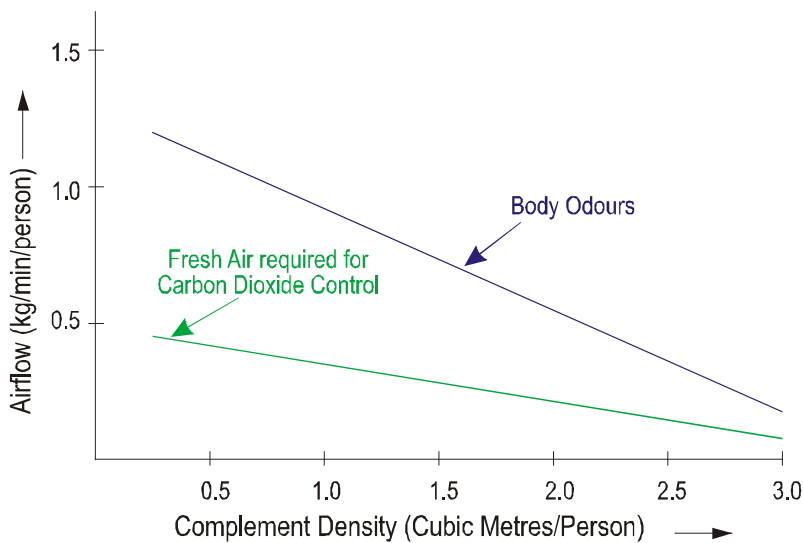
4-5 Fig 4 Ventilation Flow Requirements
