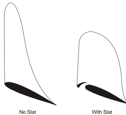
1-10 Fig 2 Effect of Slat on the Pressure Distribution
