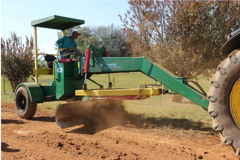
FIGURE 6.4 – RSA MANUFACTURED TOWED GRADER WITH SCARIFIER ATTACHMENT
