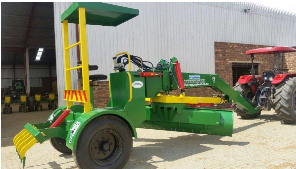
FIGURE 6.4 – RSA MANUFACTURED TOWED GRADER WITH SCARIFIER ATTACHMENT
