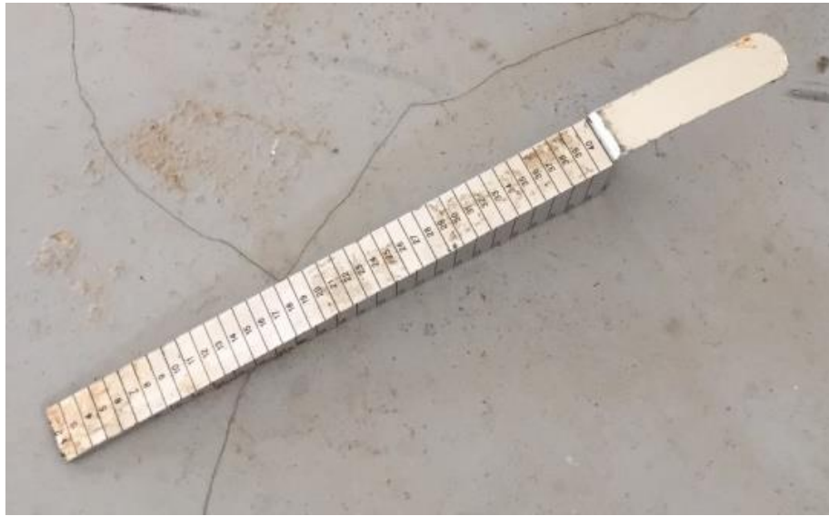
Figure 6: Calibrated aluminium wedge for rut depth measurement
