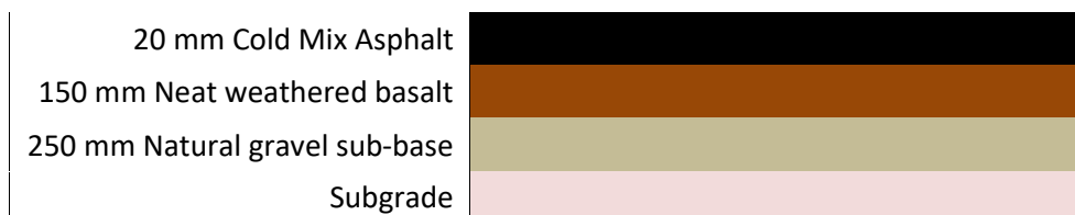
Figure 5-2: Designed pavement structure (D435)
