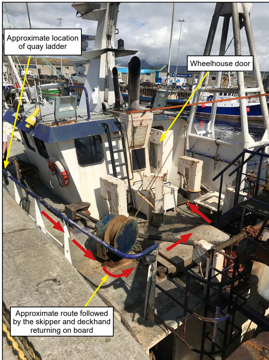
Figure 2: Access from the upper deck to the wheelhouse door
