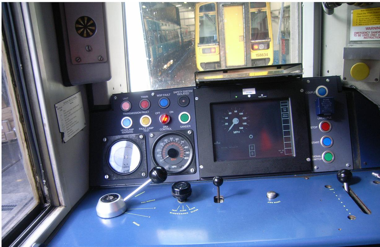
Figure 2: Typical driving cab layout and driver machine interface (DMI) screen
