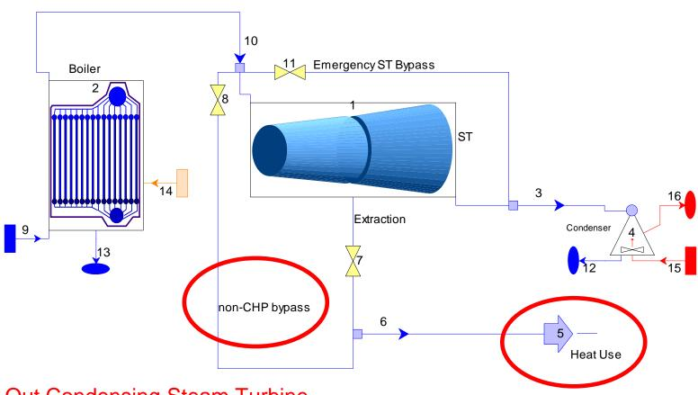
Pass Out Condensing Steam Turbine with non-CHP heat in bypass
