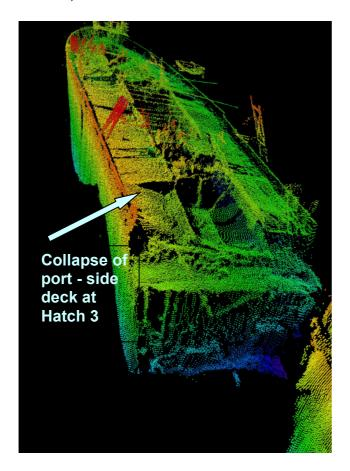
A section of the deck along the port side of Hatch 3, has collapsed. This is also evident from the 2002 survey, but appears to be more pronounced in the 2005 survey.
