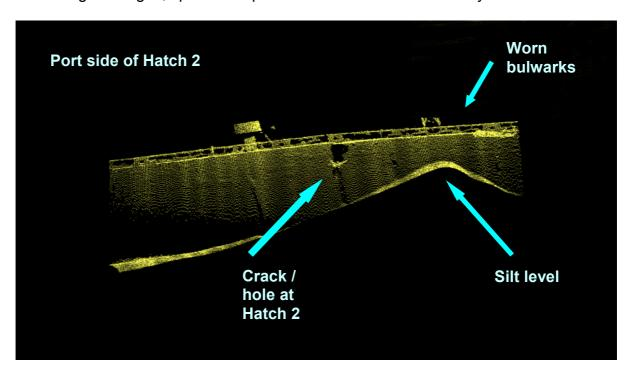
The relatively thin plating of the bulwarks is corroded all around the wreck, and numerous apertures in the main deck and on the boat deck are evident. These are likely to be constructed of thinner steel than the 5/8" (15.5mm) of the hull plating, but even here, where the hull form provides strength to the whole structure, there is evidence of corrosion in the irregular shape of most apertures and edges to splits.
