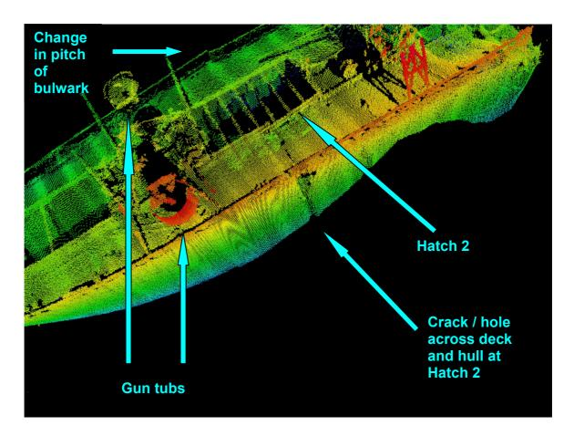
Distortion is apparent in the bow section, probably owing to the weight of cargo, and this is especially noticeable in Hold 2. On the starboard side this has resulted in a longitudinal crease in the hull plating at 'tween deck level running for 11m from a major split to the aft end of Hold 2. Below this the side of the ship just above the turn of the bilge has been pushed outboard by up to 2m. Forward of the split there appears to be a 4m long aperture just detectable at the turn of the bilge.
