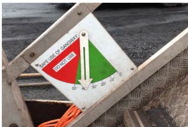
Figure 4 Inclinometer on a gangway
