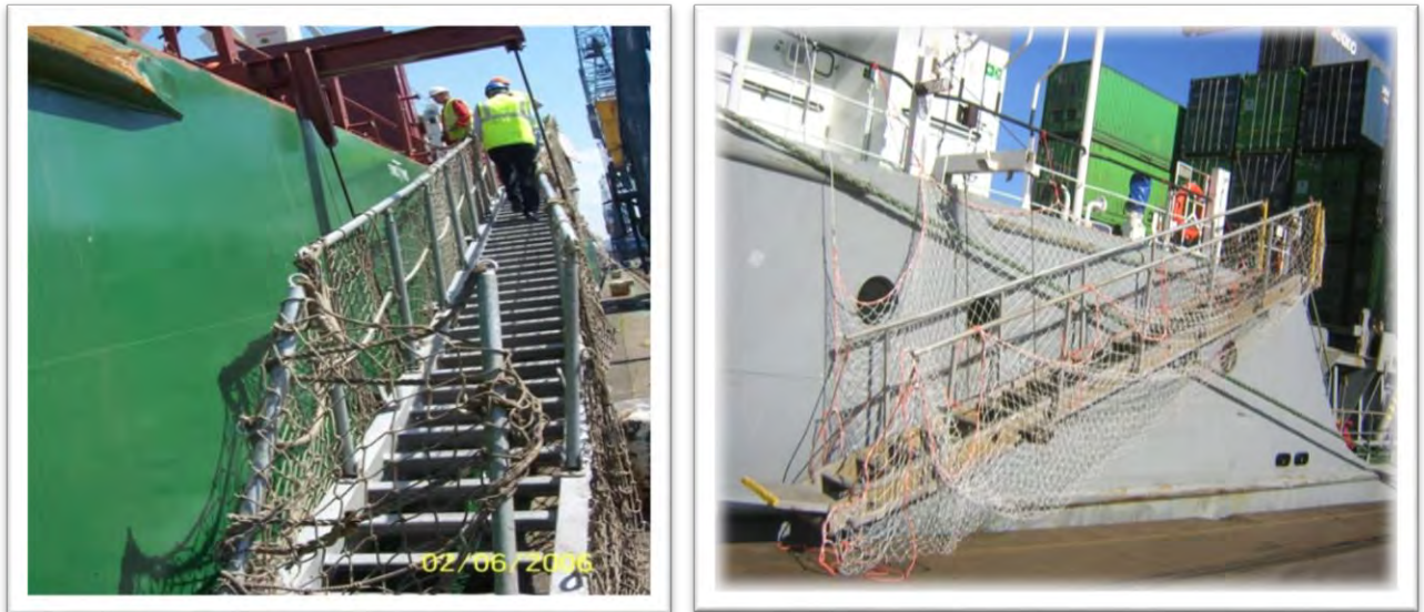
Figure 3 Accommodation ladders with safety nets deployed
