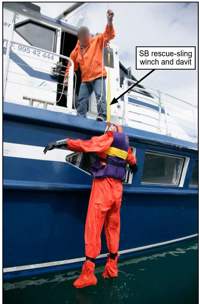
**Figure 7c:** SB rescue-sling in use
