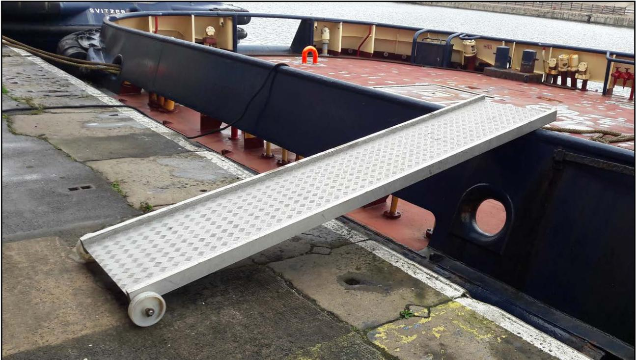
**Figure 11:** Ramp used in gangway trial
