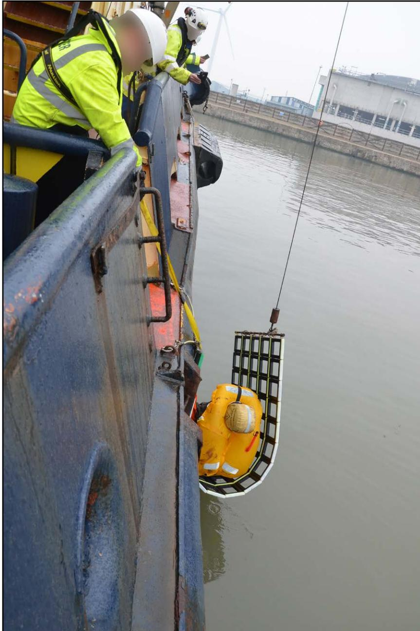
**Figure 8:** Jason's Cradle equipment being used during a drill
