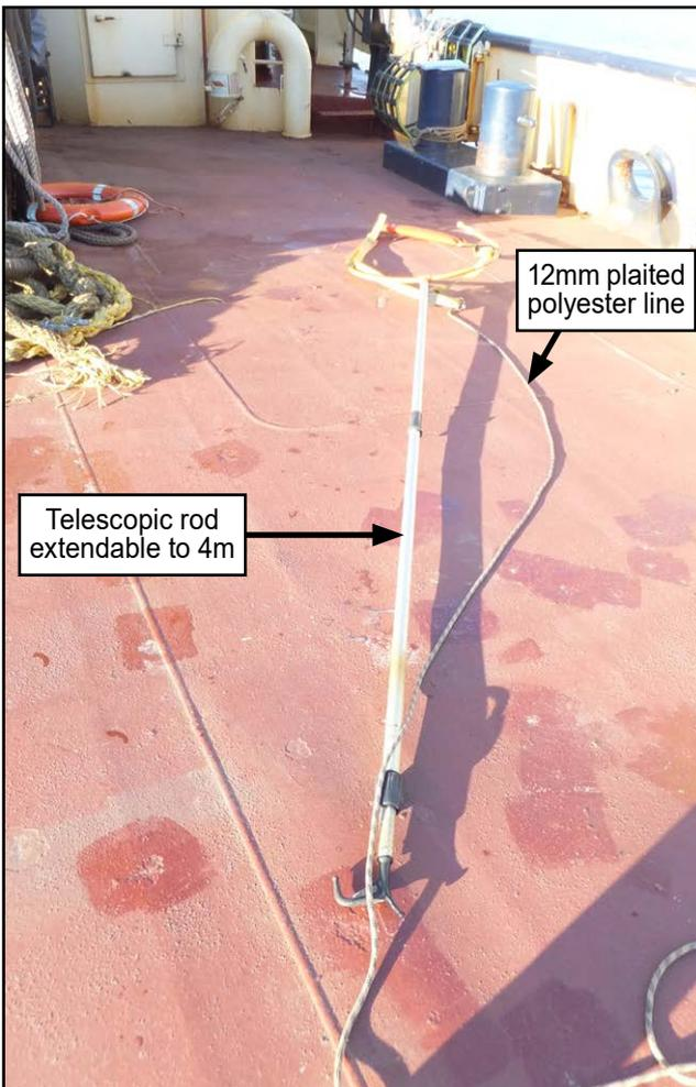
**Figure 7b:** SB rescue-sling with extended handle
