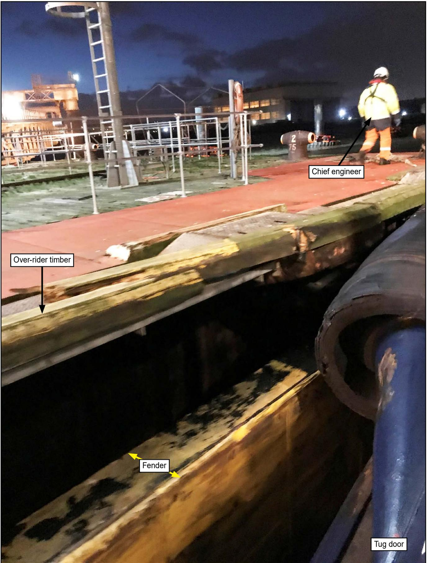
**Figure 4:** Chief engineer on north oil stage about to release the head line (photograph taken by a crew member to record damage caused to over-rider timber)
