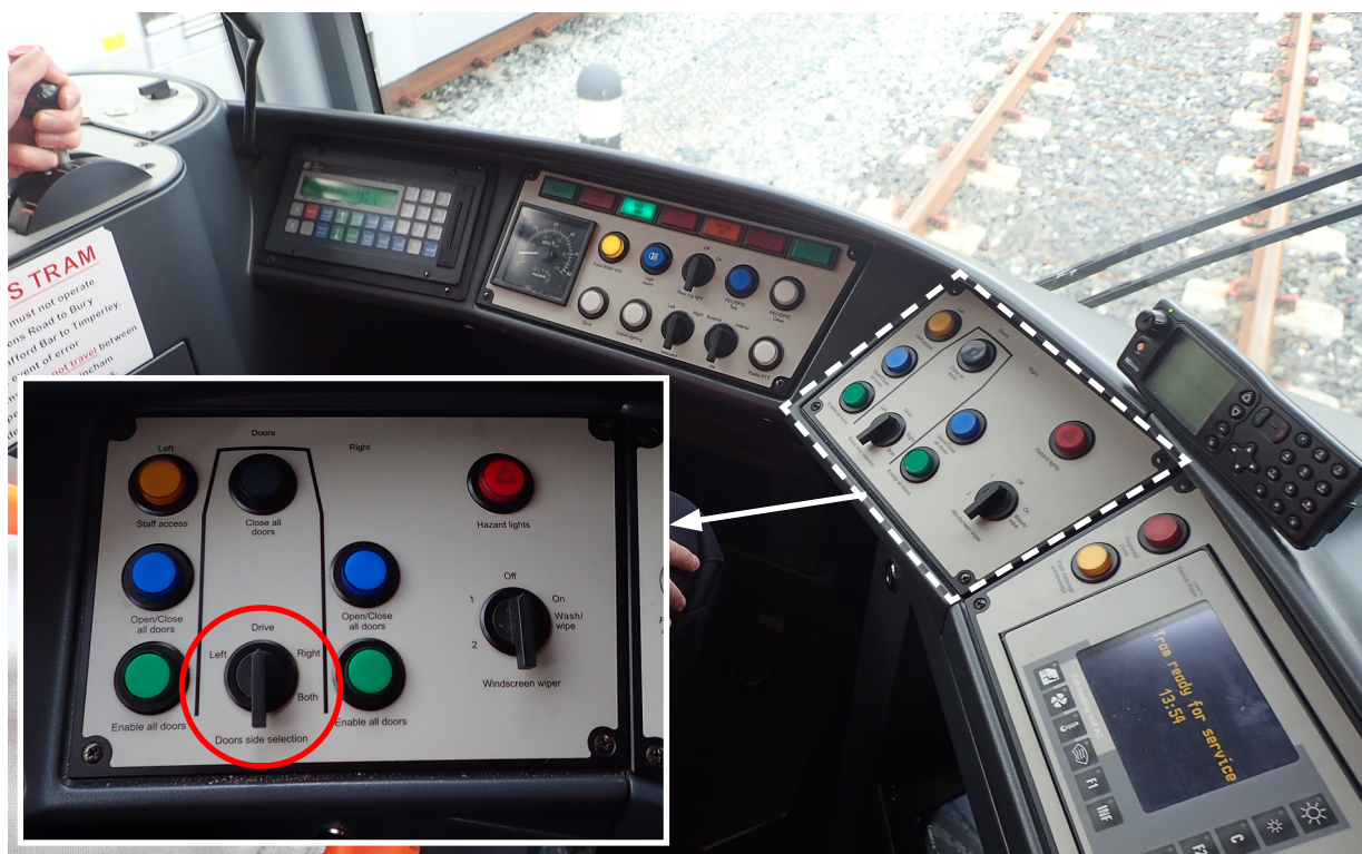
Figure 7: The door side selector switch on the driver's console
