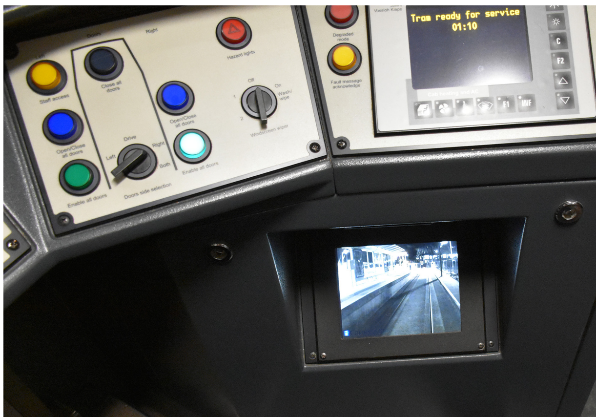
Figure 10: positioning of rear-facing camera monitor screen
