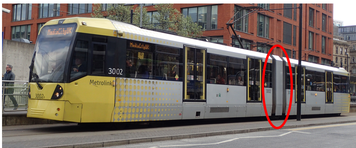
Figure 4: Photo of an M5000 tram similar to that involved in the accident, with the articulation section indicated
