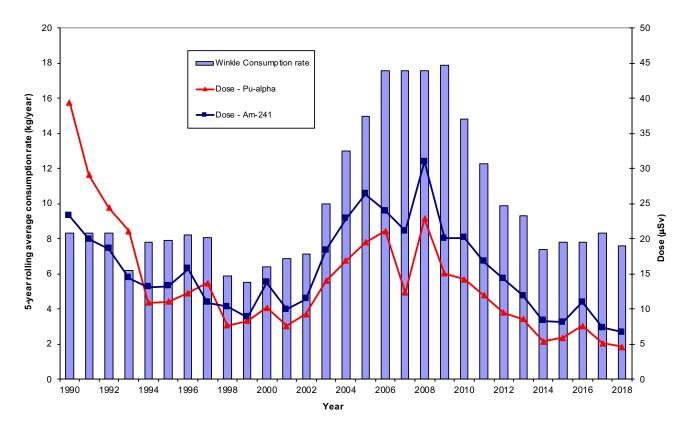
Figure 2. Dose to marine critical group from Pu-alpha and Am-241 in mussels and consumption rate
