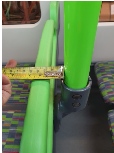
Figure 6: Vertical handrail adjacent to seat handhold
