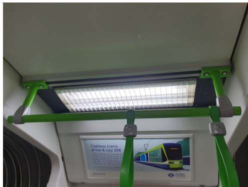
Figure 4: Horizontal handrail in C module – 1
