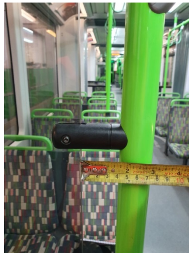
Figure 7: Draft screen vertical handrail
