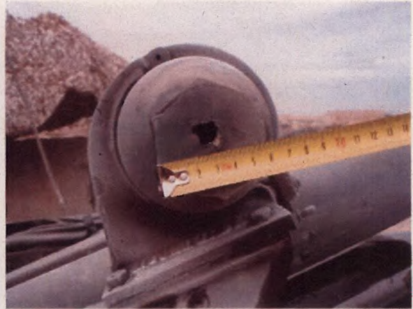
Figures 5 / 5a – Recuperator reservoir left and right end screwed plugs
