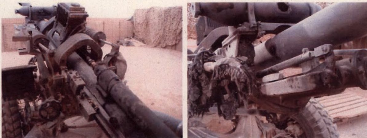
Figure 2 – Fire and smoke damage
