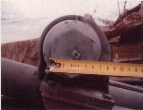
Figures 5 / 5a – Recuperator reservoir left and right end screwed plugs
