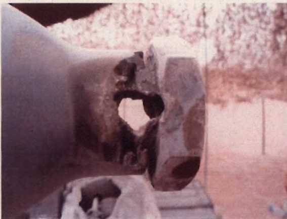
Figures 6 / 6a – Recuperator reservoir left and right sealing washer areas
