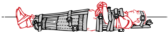
Figure 1.80 Strapped up – the arms can be strapped inside or outside the chest section of the stretcher, depending upon the injuries.
