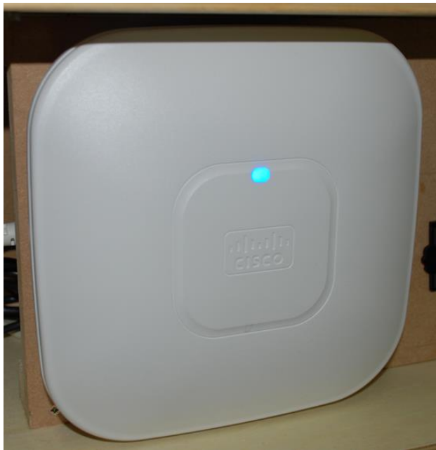
Figure 8 - Example of the Wireless Access Point (WAP)
