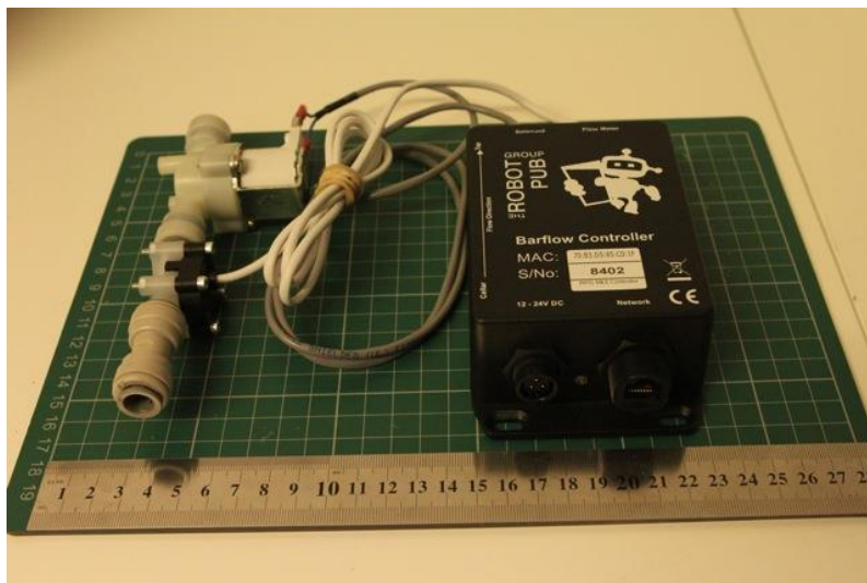
Figure 12 - Authorised alternative single input/output Barflow Controller (Mk3)
