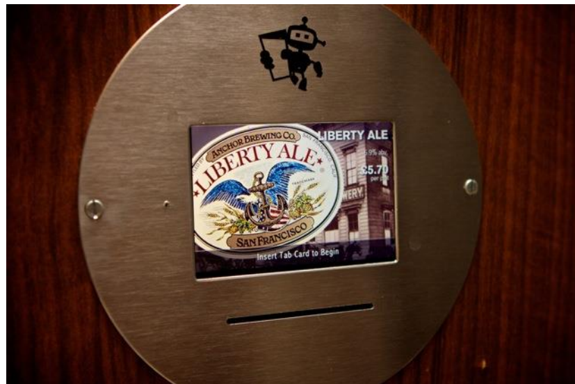
Figure 14 - Authorised alternative customer LCD touch panel and RFID card reader slot
