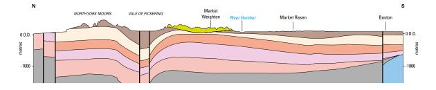
Figure 5Schematic-cross section west to east through the Eastern England region. Line of section is shown in Figure 3. Note<br/>that the vertical scale is greatly exaggerated and actual dips of rock layers are much gentler than they appear here.<br/>See Figure 2 for the key to the rock types shown.
