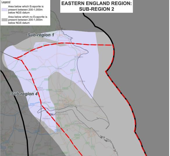
Figure 1c The areas of the Eastern England subregion 2 where Evaporite Rock Types of Interest are present between 200 and 1,000 m below NGS datum.
