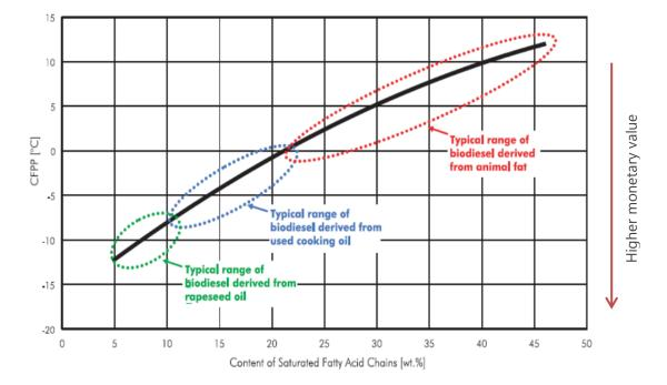
Figure 15. Relationship between cold filter plug point (CFPP) and fatty acid content for different types of biodiesel [78].
