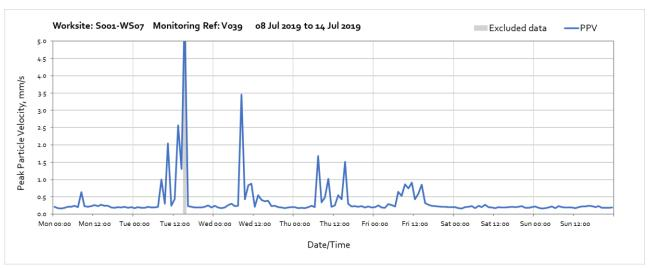
Note: High vibration levels at 15:00 on Tuesday 9<sup>th</sup> of July were due to local disturbance of the vibration monitor and are not representative of HS2 vibration levels.
