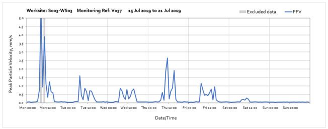
Note: High vibration levels at 08:00 and 10:00 on Monday 15<sup>th</sup> July were due to local disturbance of the vibration monitor and are not representative of HS2 vibration levels.
