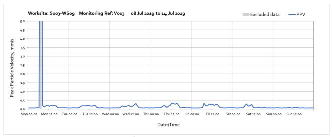
Note: High vibration levels at 07:00 on Monday 8<sup>th</sup> of July were due to local disturbance of the vibration monitor and are not representative of HS2 vibration levels.
