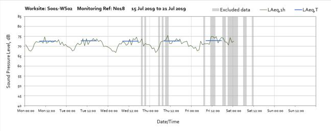
Note: Missing data between 01:00 Saturday 20<sup>th</sup> and 10:00 on Friday 26<sup>th</sup> of July was due to electrical fault at the lamp post to which the monitoring station is connected.
