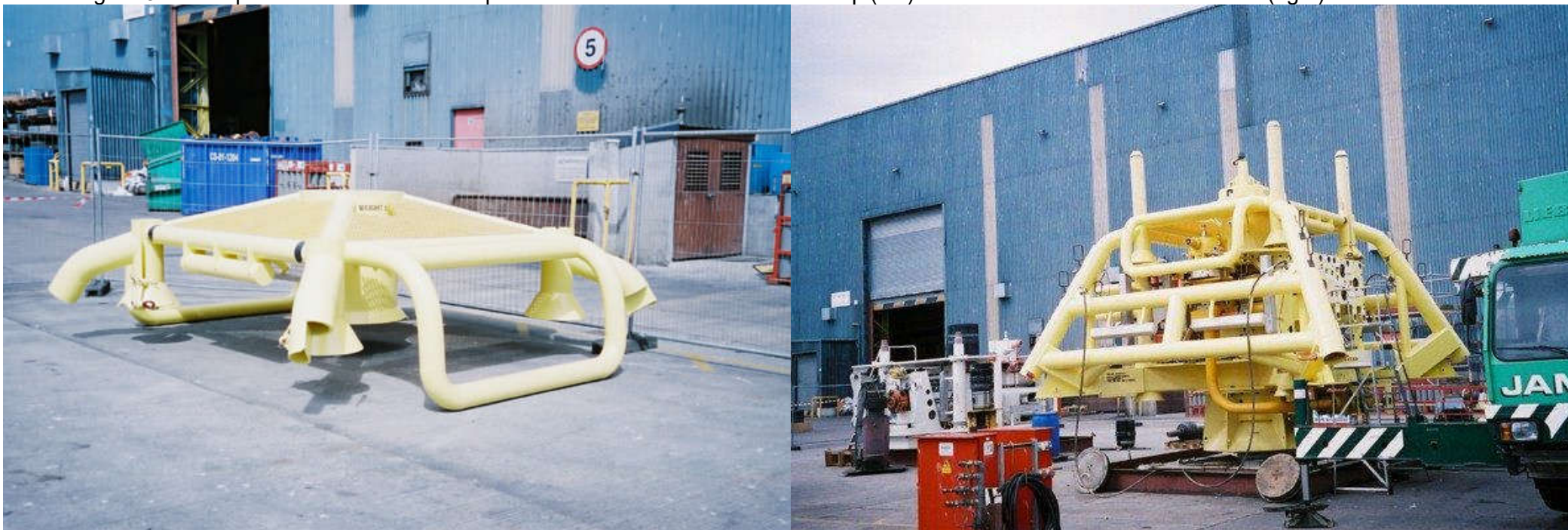
Figure 3.4: Two part WHPS and debris cap structure on subsea well - debris cap (left) and WHPS on wellhead Xmas tree (right)
