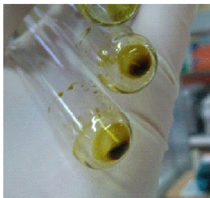
Figure 5. Reconstituted black pepper QuEChERS extracts after spin filter (0.2 µm) centrifugation. From left to right, water/methanol/acetonitrile (v/v): 1/3/0, 1/1/0, 3/1/0, 2/1/1, 1/1/2
