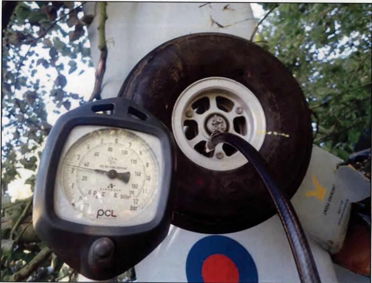
Figure 12: Main wheel tyre pressure check.
