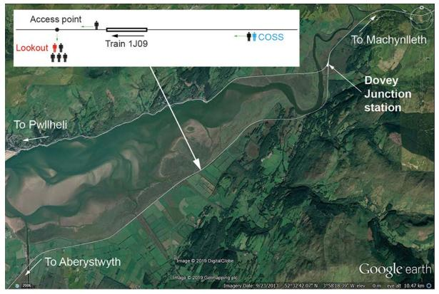
Track layout showing the location of the incident, the direction of the train and the approximate position of the work group at the time of the incident
