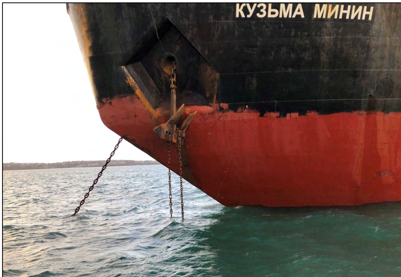
Figure 2: Port anchor fouled by chain
